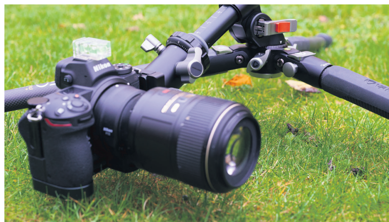
ABOVE Fit an L-grip on your camera and the 263CB with its MACC means you can get your camera almost to ground level
